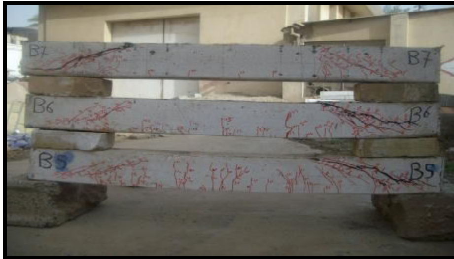
Figure (5): Crack Patterns for Fibrous Beams B5, B6 and B7.
