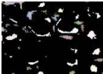
Fig 7:Wear Debris as Metallic and Oxidative Particles at 7.5 m/min, 195 KN/m 2 & 6 minutes X20
