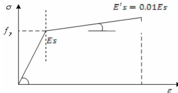
Figure 3: Elastio-plastic stress-strain relationships for steel(Xiong, and Zha, 2007)
