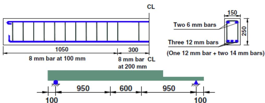
**Figure 8:** Reinforcement details of the concrete beam specimens (dimensions :mm)
