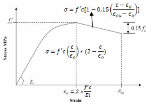
**Figure 1 :** Uniaxial stress-strain of concrete in compression(Hognestad, 1951).
