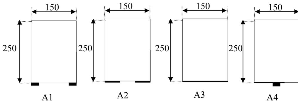
**Figure 11:** The locations of prestressed CFRP plate.
