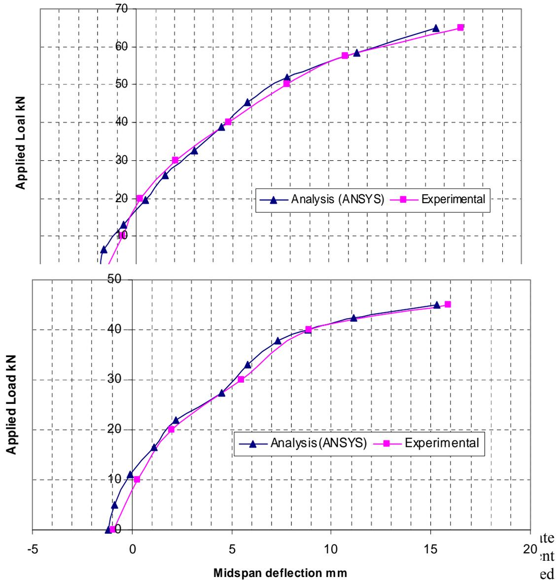
CFRP plate give minimum deflection under same load and in the same time has maximum load capacity. For this purpose many locations of CFRP plate are investigated and with different width and thickness of prestressed CFRP plate as listed in table (4)
