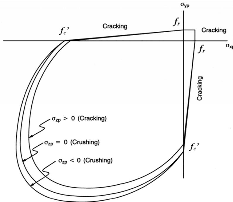
Figure 2: 3D-failure surface for concrete (ANSYS, 2006).
