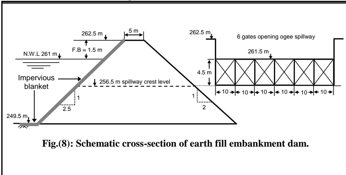
**Fig.(8): Schematic cross-section of earth fill embankment dam.**
