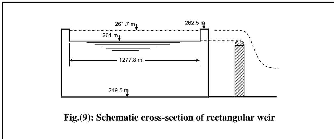
**Fig.(9): Schematic cross-section of rectangular weir**
