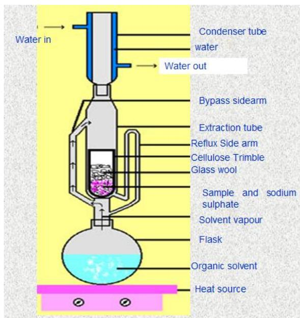
**Fig. (2) Soxhlet apparatus used for extraction process.**
