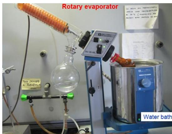
**Fig. (3) Rotary evaporator used for evaporation.**
