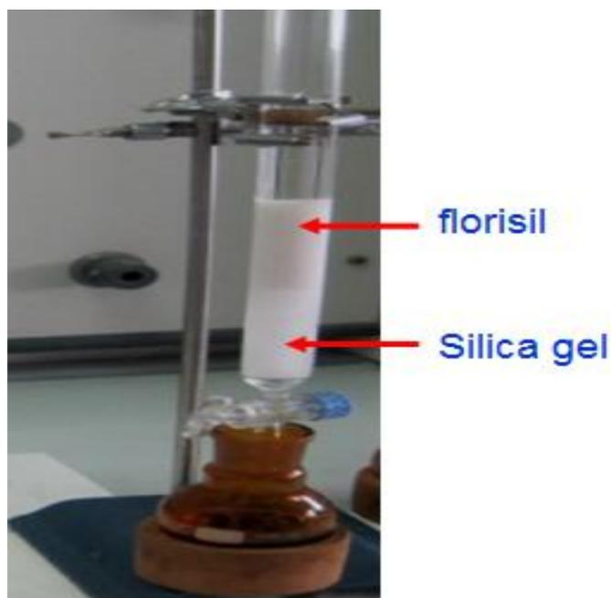
*Fig.(5) Purification by chromatographic column*
