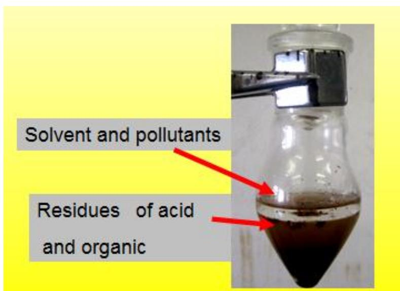
**Fig.(4) Heart shaped flask used for acid digestion.**
