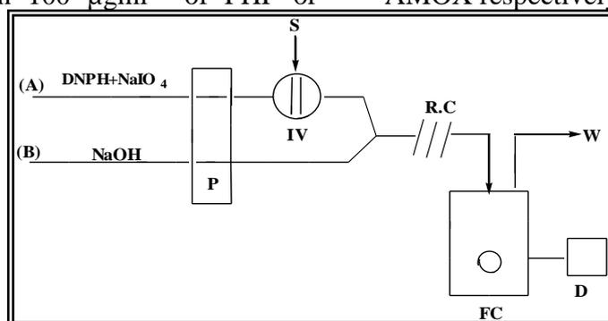
**Fig.(2) Manifold employed for FIA-Spectrophotometric determination of PHP and AMOX with DNPH and sodium periodate solution in alkaline medium where: IV, Injection valve ; R.C., Reaction Coil ; S , Sample ; P, Peristaltic pump ; FC , Flow cell ; D, Detector ; W, Waste.**
