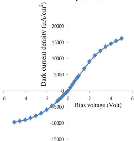
**Fig.2: J-V characteristic curve of (Al/Psi/n-Si/Al) of etching time (40 minute)**
