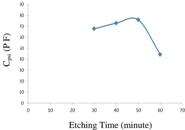
**Fig.5: The capacitance of porous silicon function of time etching**
