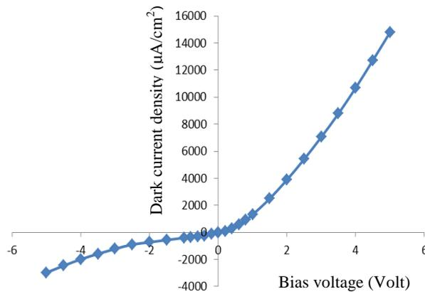
**Fig.4: J-V characteristic curve of (Al/Psi/n-Si/Al) of etching time (60 minute)**
