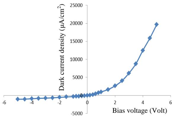
**Fig.3: J-V characteristic curve of (Al/Psi/n-Si/Al) of etching time(50 minute)**
