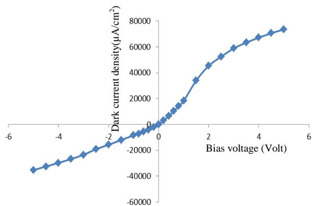
**Fig.1: J-V characteristic curve of (Al/Psi/n-Si/Al) of etching time (30 minute)**
