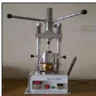
**Figure 4: Plastic injection machine**
