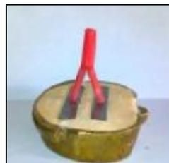
**Figure 2: Wax sprue on top of metal pattern**
