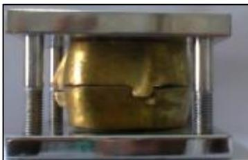
**Figure1: Nylon flask in the clamp**
