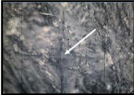
**Figure 1: Surface Micro-Hardness indentation**
