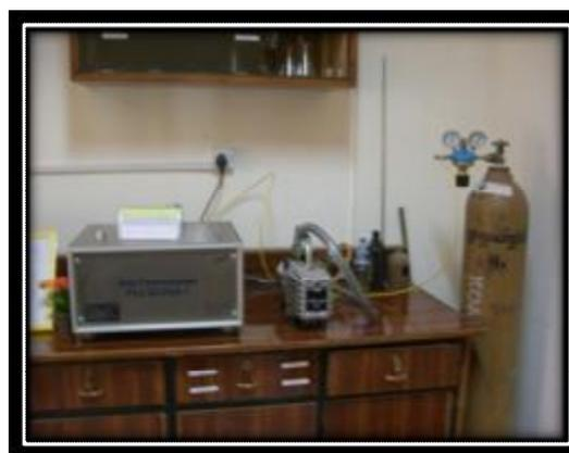
**Figure 3: Gas helium pycnometer machine**
