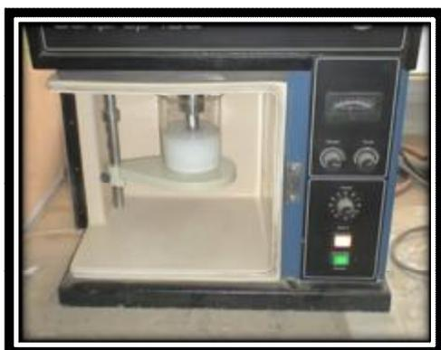
**Figure 2: Probe sonication apparatus**
