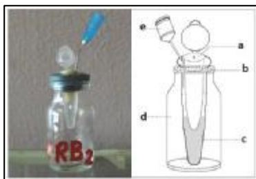
Figure 1: (a) Root. (b) Rubber stopper. (c) Eppendorf tube. (d) Glass vial. (e) 27 gauge needle.
