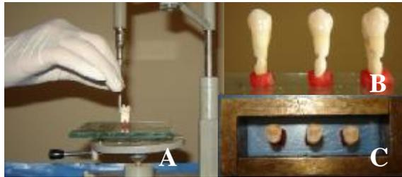
**Figure 2:** A, fitting of the tooth on a glass slab with a soft sticky wax, analyzing rod of the surveyor was used to align the middle third of the buccal surface. B, three teeth were aligned on the glass slab, retentive wedge shaped cuts were made along the sides of the roots of each tooth. C, the two L-shaped metal plates placed opposite to each other to form a box around the teeth.
