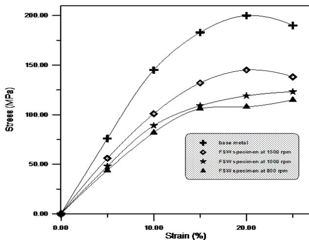
Fig(4) Tensile test results for base metal , FSW specimens at : 1500 rpm , 1000 rpm and 800 rpm
