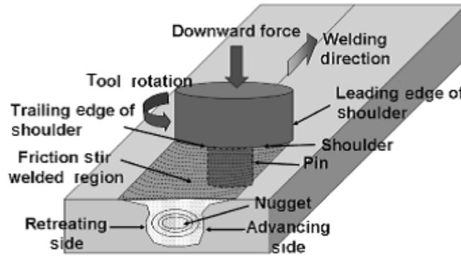
Fig. ١ Friction stir welding process <sup>[١]</sup>
