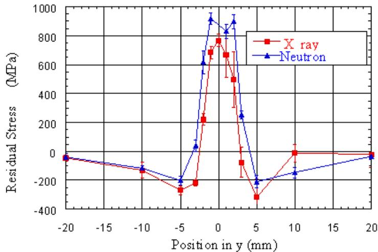
The behavior of residual stress in Fig(10) similar to behavior of hardness value distribution as shown in figure(9) to figure(9) ,That the change in the value of hardness resulting from the change in the value of the heat transmitted generated as a result of the speed of revolution of the pin and show that the values of hardness near the welding line is low then rise and then begin to decreasing gradually and
