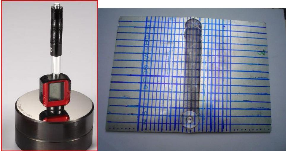
Fig(3) Leeb hardness device and meshing stir welding specimen
