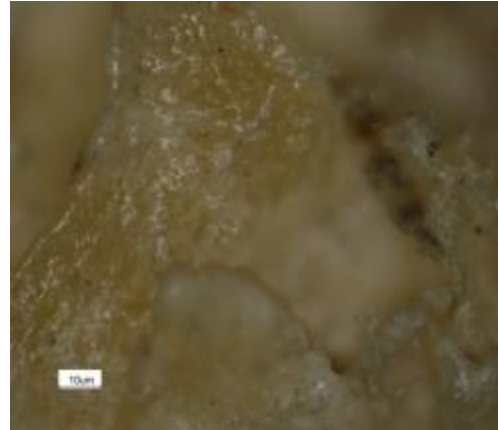
Figure (2) Optical Surface Microstructure of 15% Ben. (70µm particle size).
