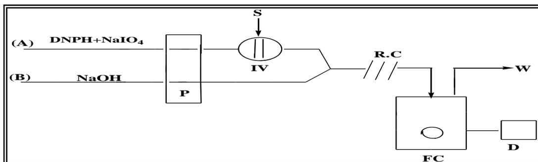
**Figure 1-** Manifold employed for FIA-Spectrophotometric determination of SLB and PYD with DNPH and sodium periodate solution in alkaline medium where: IV, Injection valve ; R.C, .Reaction Coil ; S , Sample ; P, Peristaltic pump ; FC ,Flow cell ; D, Detector ; W,Waste.
