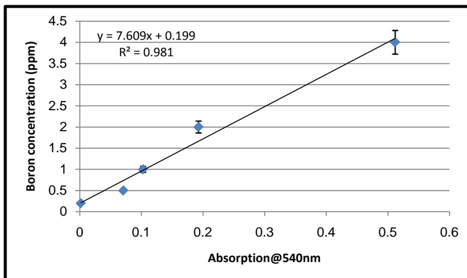
**Figure-3. The calibration curve – Boron**
