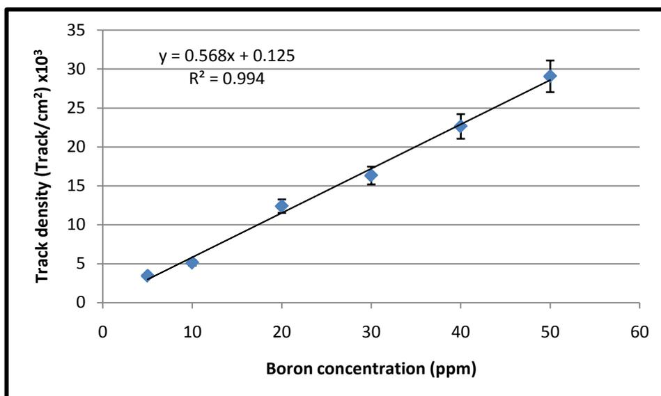
Figure-2. The calibration curve – Boron
