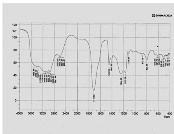
**Figure 1-** FTIR spectra of Poly acrylic acid .
