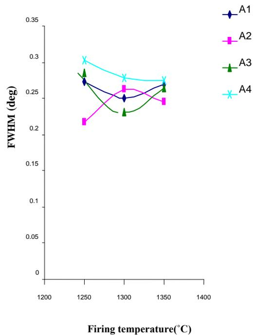
**Figure 4-** X-ray line broadening (FWHM) with firing temperatures.
