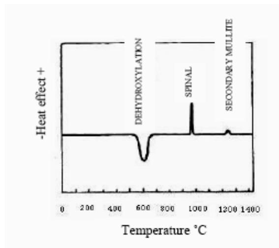
**Figure 3-** Differential thermal analysis curve for pure well crystallized kaolin[9].
