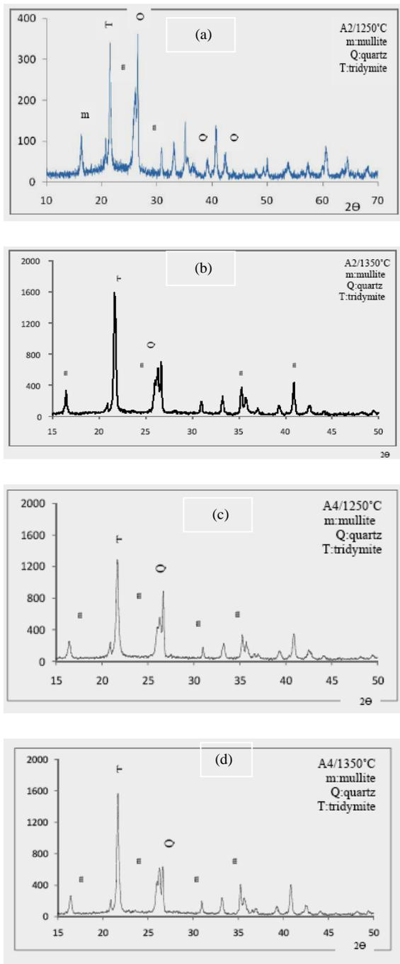
**Figure 5-** (a-d) XRD patterns for the fired samples A2 and A4 at 1250°C and 1350°C for two hours
