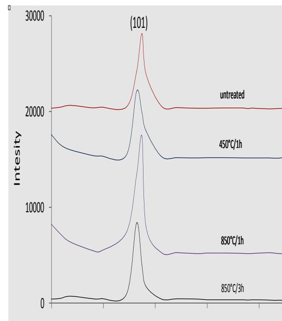
**Figure 2-** Illustration of X-ray line broadening for calcinated kaolin.
