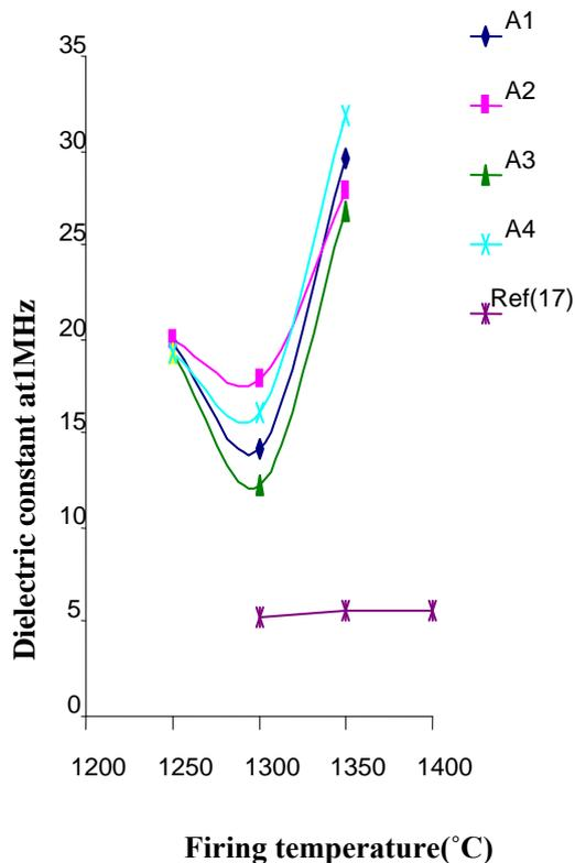
**Figure 7-** Dielectric constant at 1MHz corresponding to Firing temperature.
