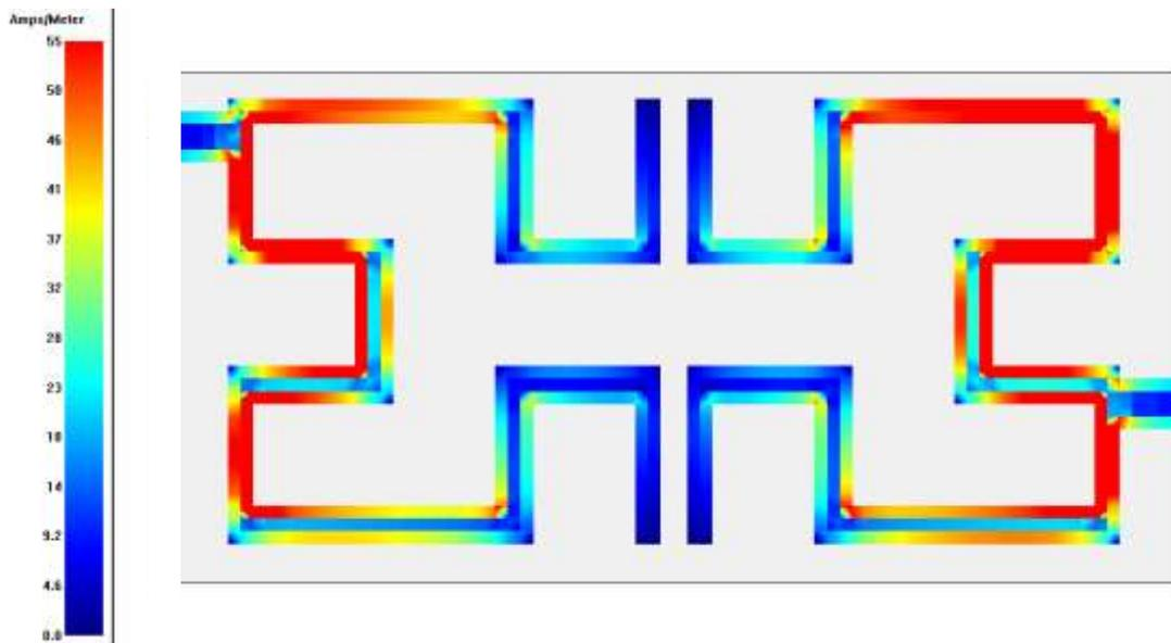
Figure(8) Current density distribution at the conducting surface of the 2<sup>nd</sup> iteration stubbed Hilbert bandpass filter simulated at a resonant frequency of 2.4 GHz
