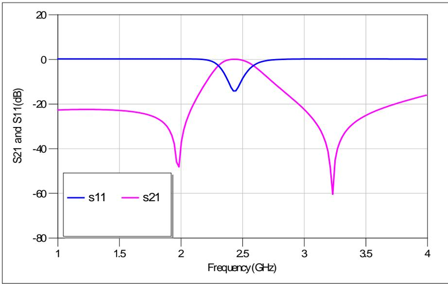
Figure.(3) The return loss ( $S_{11}$ ), and transmission ( $S_{21}$ ) responses of the filter structure based on the 3rd iteration Hilbert curve geometry depicted in Fig.(2)
