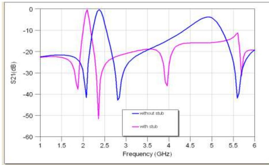
Figure.(7) The out-of-band transmission responses of the proposed filters based on the 3rd iteration Hilbert curve geometry; with and without stubs.
