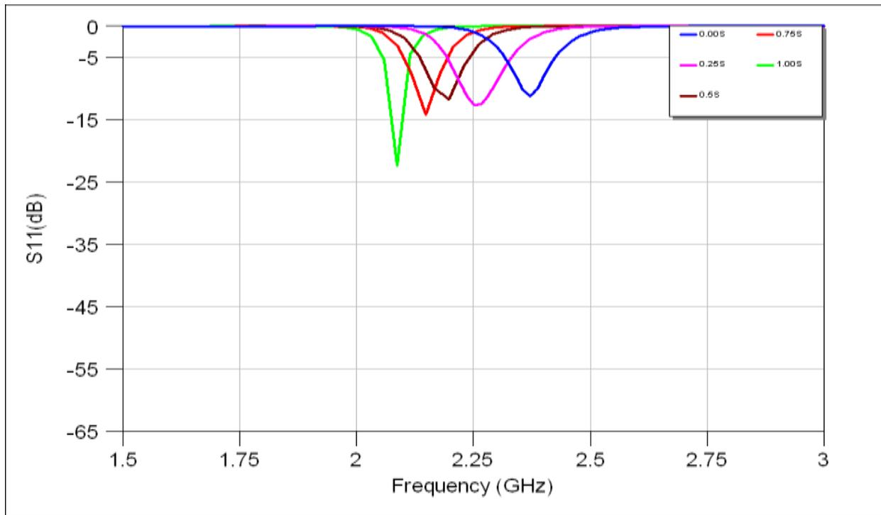
Figure.(6) The return loss responses ( $S_{11}$ ) of the filter structure based on the 3rd iteration Hilbert curve geometry with stub depicted in Fig.(4)
