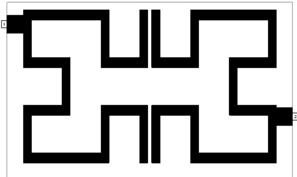
Figure.(2) The layout of the two-pole microstrip bandpass filter based on the 2<sup>nd</sup> iteration Hilbert curve geometry
