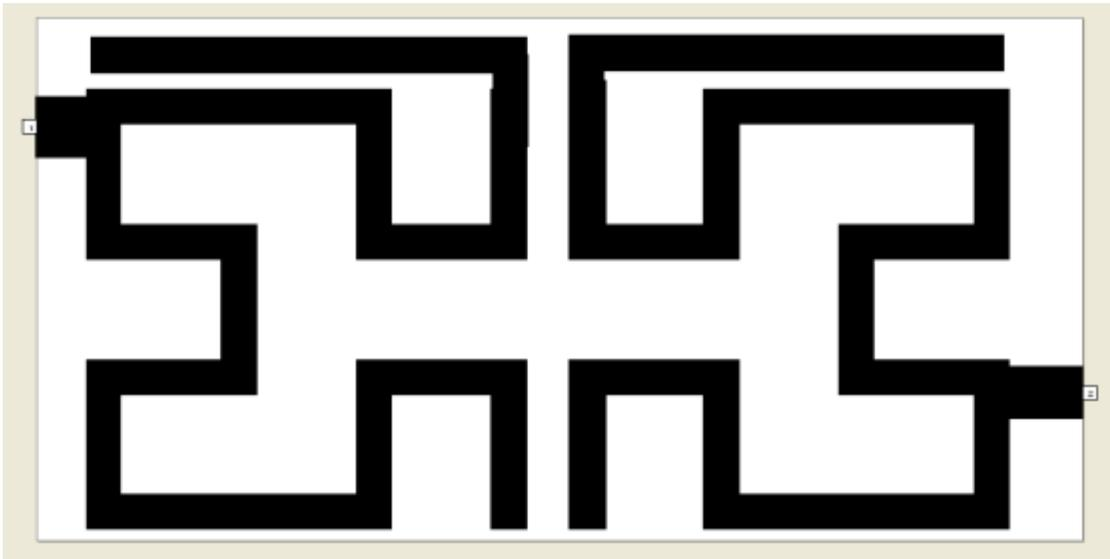
Figure.(4) The layout of the modeled two-pole microstrip bandpass filter based on 2<sup>nd</sup> iteration Hilbert resonators with tuning stubs
