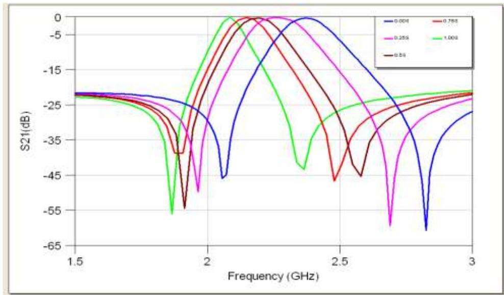
Figure.(5) The transmission responses ( $S_{21}$ ) of the filter structure based on the 3rd iteration Hilbert curve geometry with stub depicted in Fig.(4)
