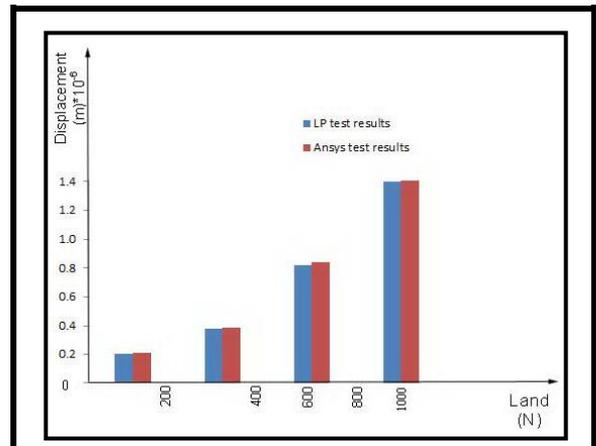
Fig. (6) Load versus displacement for LP and ANSYS tests results (ply angle  $0^\circ/90^\circ$ ).
