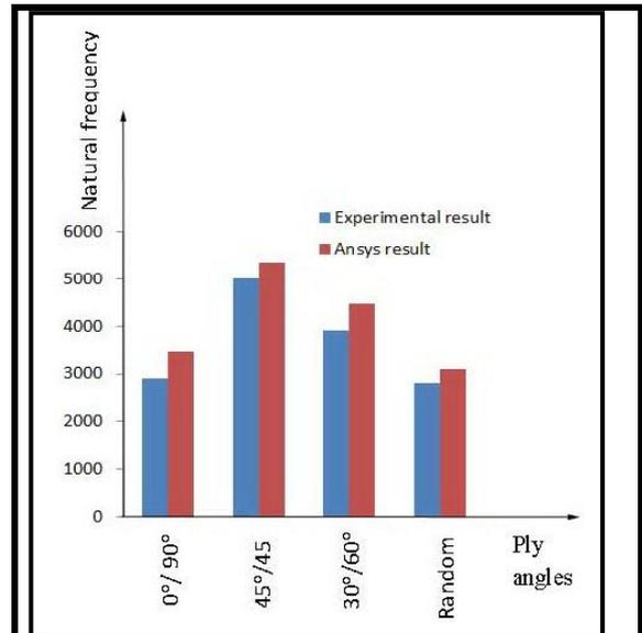
Fig.(9) Ply angles versus first natural frequency for experimental and ANSYS results of GA optimized plates. (8 layers).
