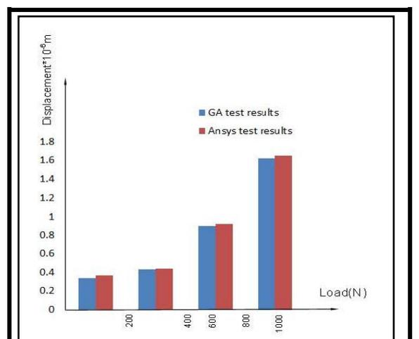
Fig.(7) Load versus displacement of GA and ANSYS tests results (ply angle  $45^\circ / -45^\circ$ ).
