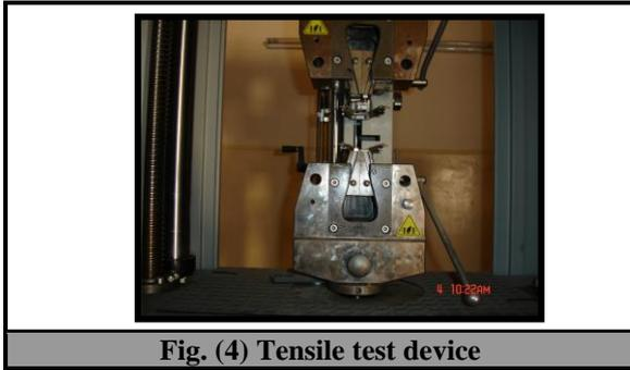
Fig. (4) Tensile test device
