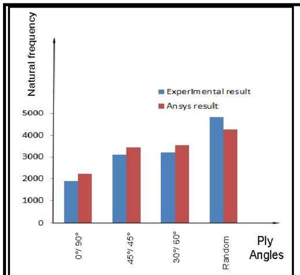
Fig.(8) Ply angles versus first natural frequency for experimental and ANSYS results of LP optimized plates. (10 layers).
