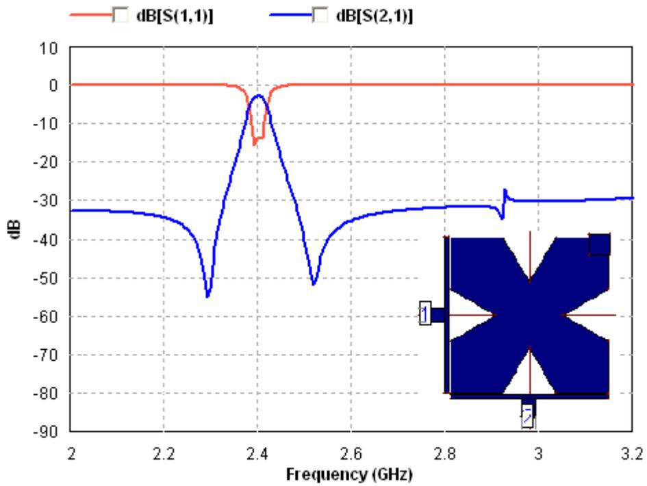
Fig.5. The return loss and transmission responses of the dual-mode microstrip square patch resonator depicted in Fig. 2c.
