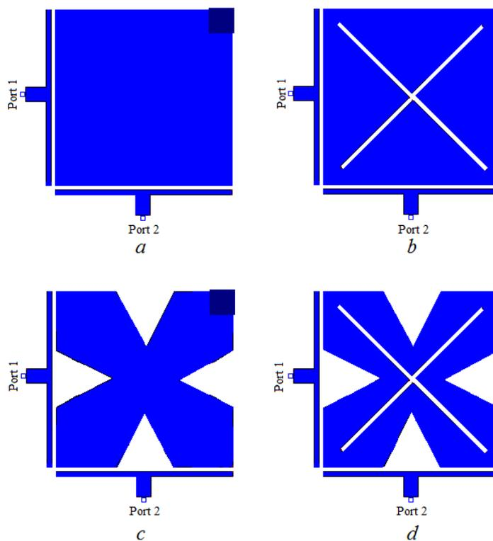
Fig.2 The layouts of the modeled dual-mode microstrip patch bandpass filters with resonators based on (a) the conventional square patch, (b) the conventional square patch and a crossed slot structure, (c) the first iteration fractal Koch curve patch, and (d) the first iteration fractal Koch patch curve and a crossed slot structure.
