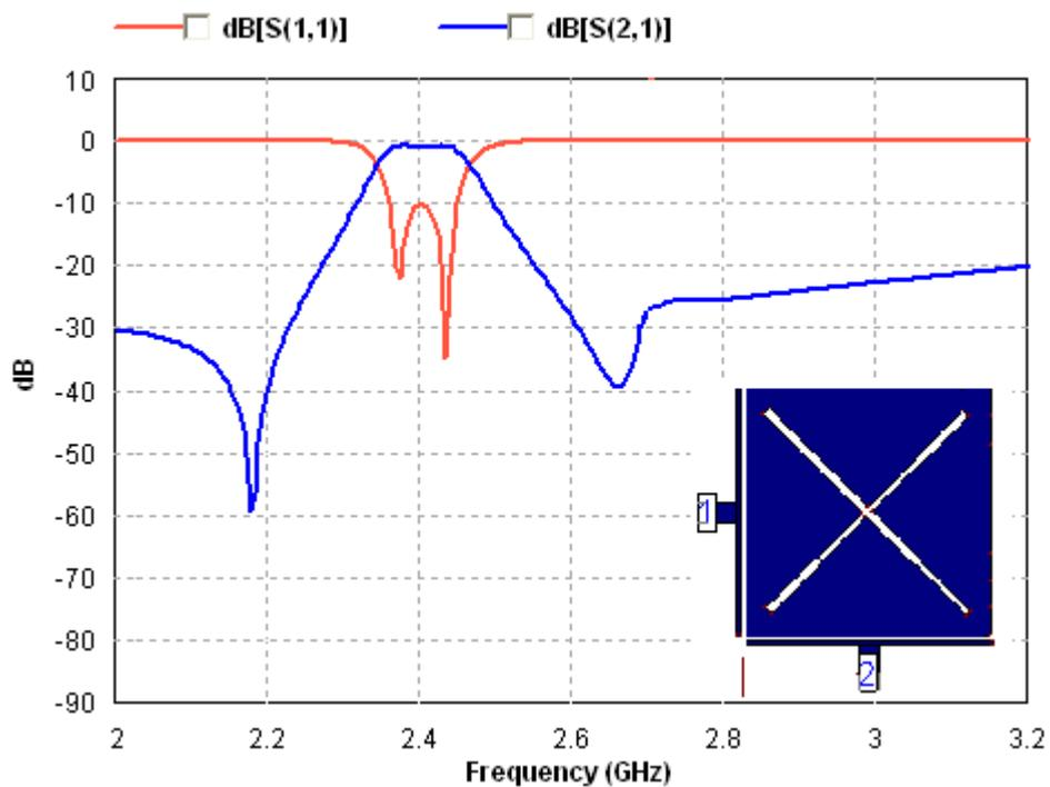
Fig.4. The return loss and transmission responses of the dual-mode microstrip square patch resonator depicted in Fig. 2b.
