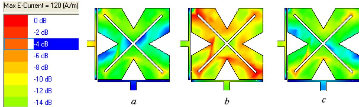
Fig. 7. Current density distribution at the surface of the first iteration microstrip bandpass filter with slots simulated at frequency of (a) 2.3 GHz, (b) 2.4 GHz, and (c) 2.5 GHz.
