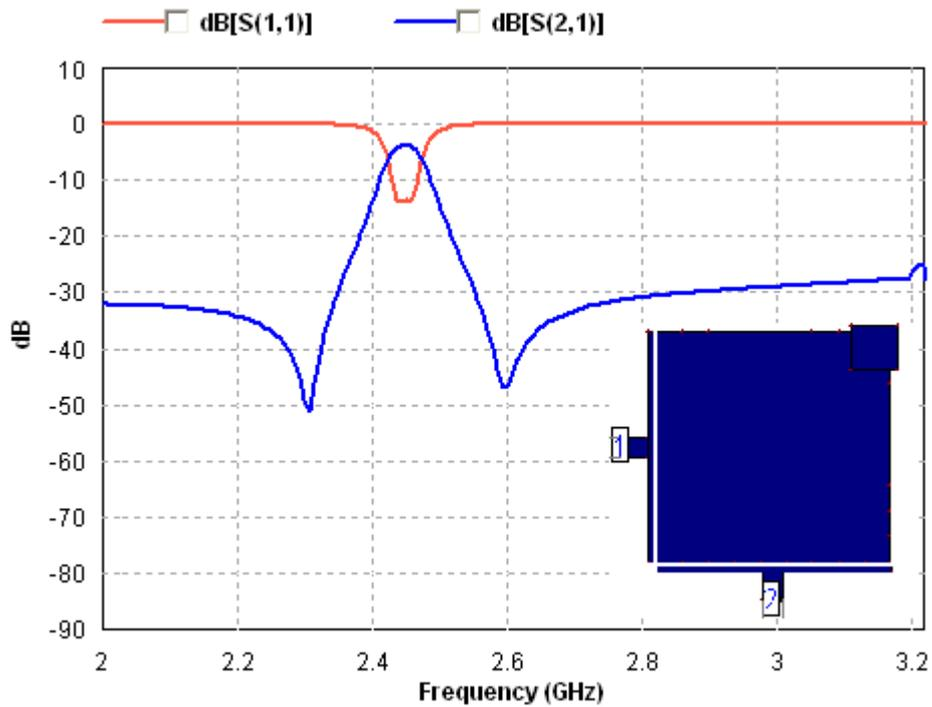
fig3.the return loss and transmission responses of the dual-mode microstrip square patch resonator depicted in Fig.2a.
