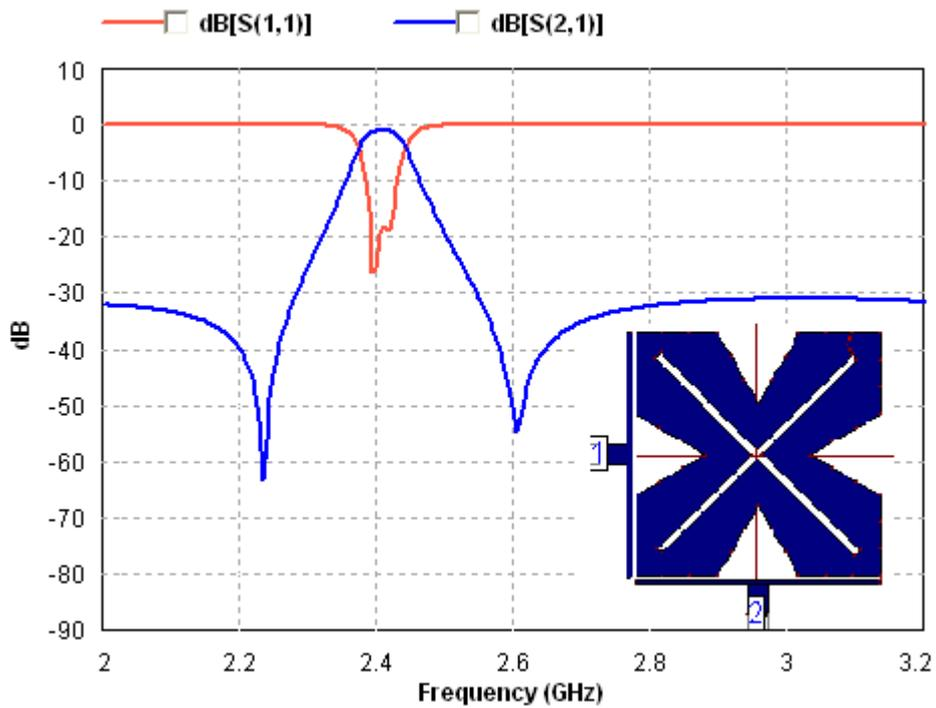
Fig.6. The return loss and transmission responses of the dual-mode microstrip square patch resonator depicted in Fig. 2d.
