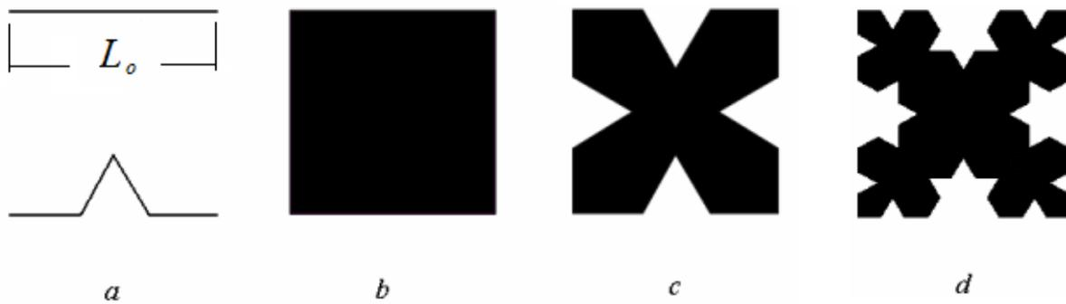
Fig.1 The generation process of the proposed fractal microstrip patch antenna structures based on fractal Koch curve. (a) the generator. (b) the initiator (square patch antenna), (c) the first iteration, and (d) the second iteration.
