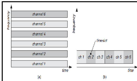
Figure 2: Frequency and Time Division Multiple Access
