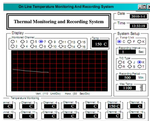
Fig ( 2): Thermal monitoring and Recording system
