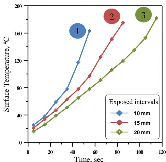
Fig (3): Thermal erosion test with different exposed intervals
