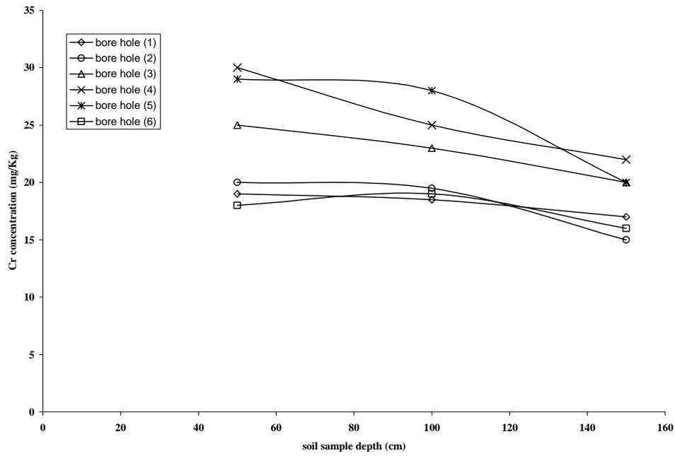
Fig (10) Concentration of Cr at various soil sampling depth
