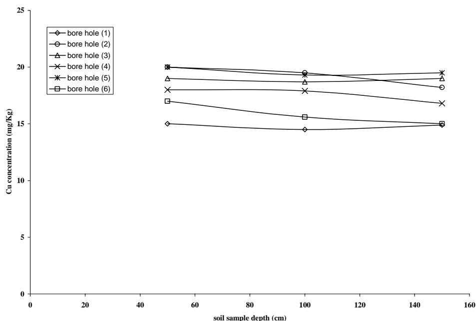
Fig (12) Concentration of Cu at various soil sampling depth
