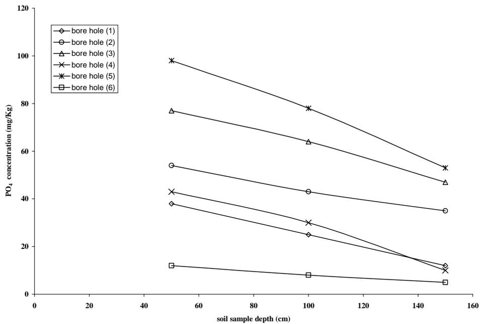
Fig (5) Concentration of PO<sub>4</sub> at various soil sampling depth
