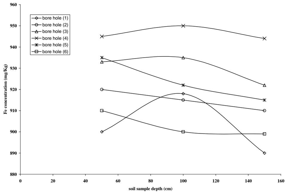
Fig (11) Concentration of Fe at various soil sampling depth
