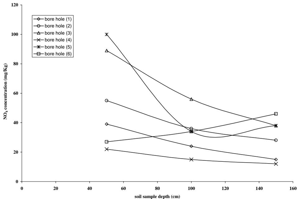
Fig (6) Concentration of NO<sub>3</sub> at various soil sampling depth
