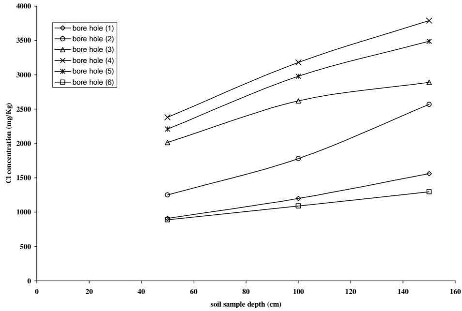
Fig (4) Concentration of Cl at various soil sampling depth
