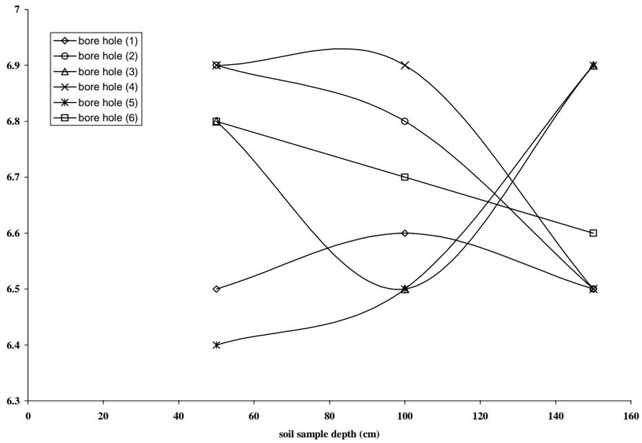
Fig (8) pH at various soil sampling depth
