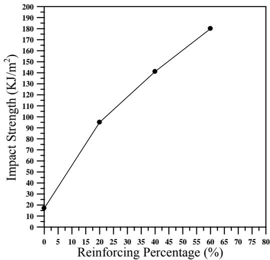
Figure(2): Impact strength versus carbon – Kevlar reinforcing percentage
