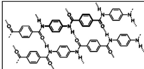
Figure (1): Chemical structure of Kevlar
