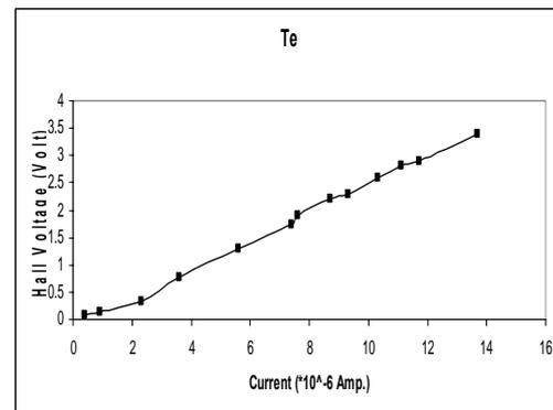
Figure 6: Variation in Hall voltage of Tellurium thin film with current.
