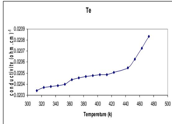
Figure 4: Variation of conductivity of Tellurium thin
