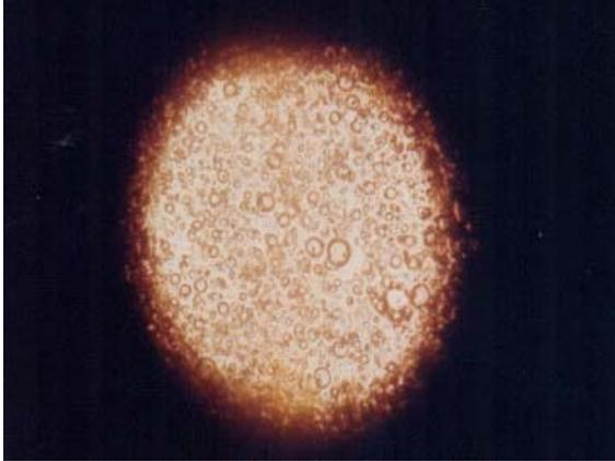
Figure 3: The topographical surface of Tellurium thin film. (x200)
