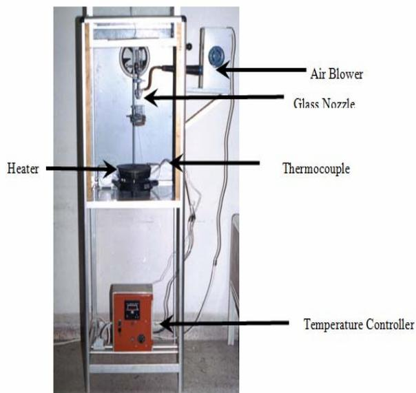
Figure 1 A photograph of the spray pyrolysis
