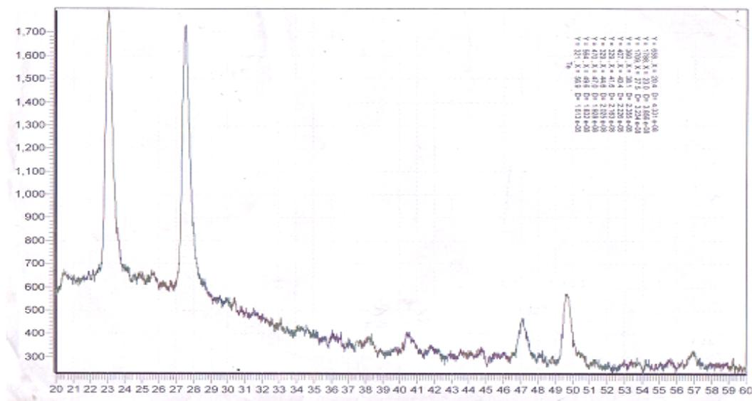
Figure 2: X-Ray diffraction of Tellurium thin film.
