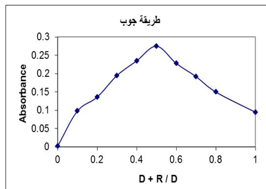
**Fig (4.) : Job's method for captopril - dichlorone product**
