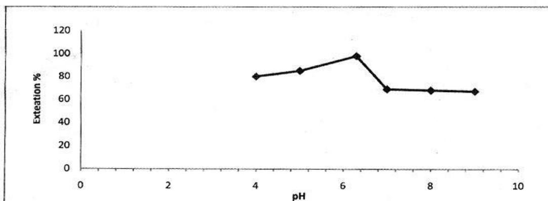
Fig ( 2) Extraction of Cu(II) as a Function of pH
