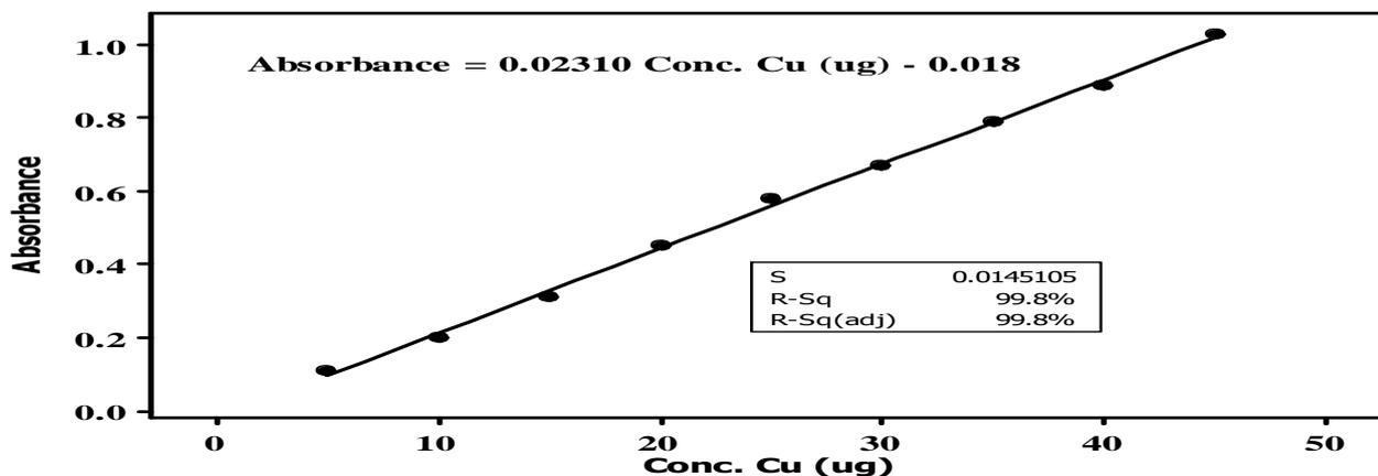
Fig (5) Calibration plot of Cu(II) DCH-18-Crown-6
