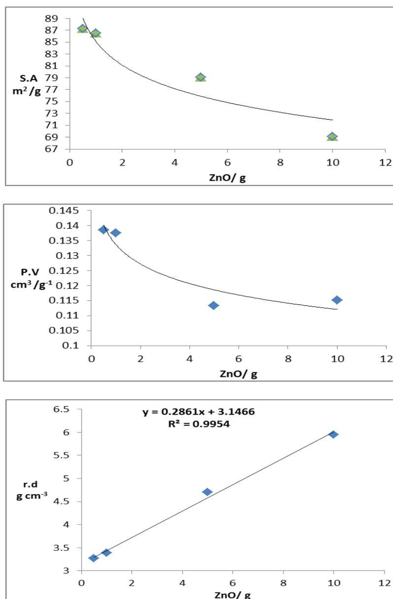
**Fig (4) Variation of (a) surface area, (b) pore volume and (c) real density with ZnO additions for modified exposed to 500 °C**
