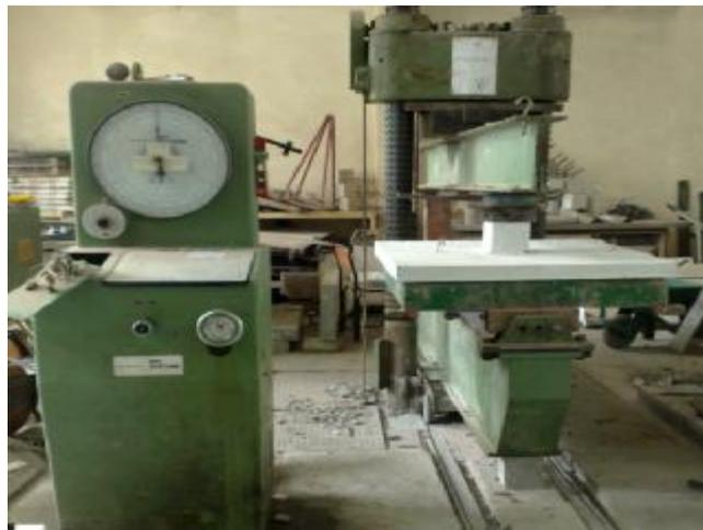
**Fig. (4) Slab Specimen Setup**
