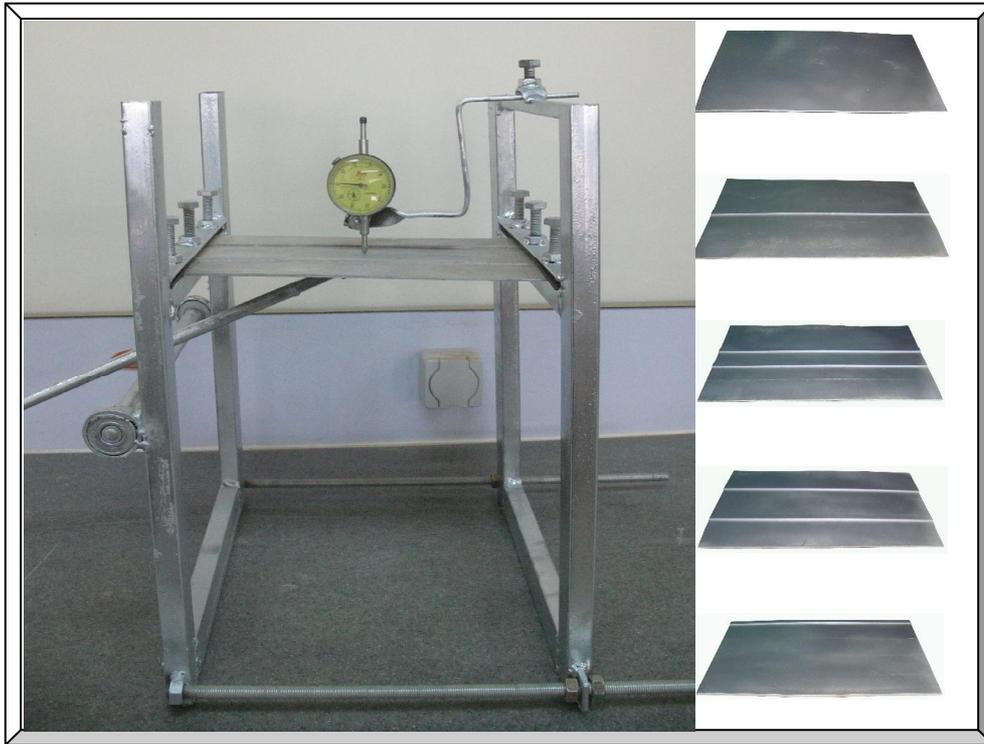
Figure (1) The constructed test rig and the test specimen's plates
