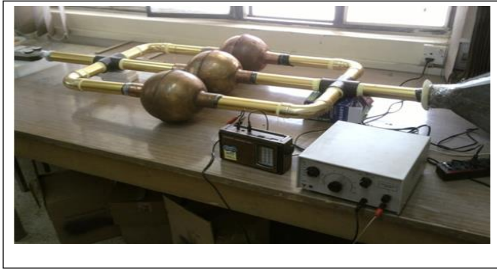
Figure (5b): Photo of spherical silencers in parallel connection.
