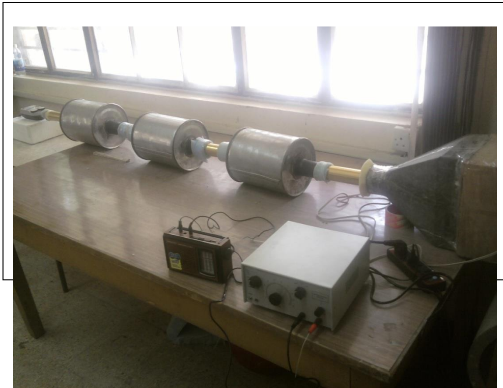
Figure (5b): Photo of spherical silencers in parallel connection.
