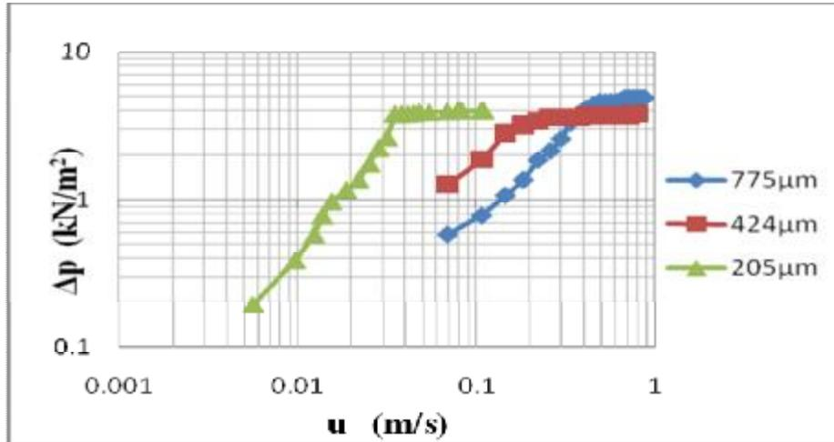
Figure (7) The relationship between the bed pressure drop and the superficial air velocity for different particles diameter, with circular baffles column,  $H_s=0.4m$ .
