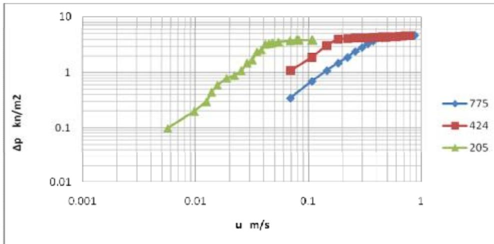
Figure (6) The relationship between the bed pressure drop and the superficial air velocity for different particles diameter, with circular baffles column,  $H_s=0.3m$ .
