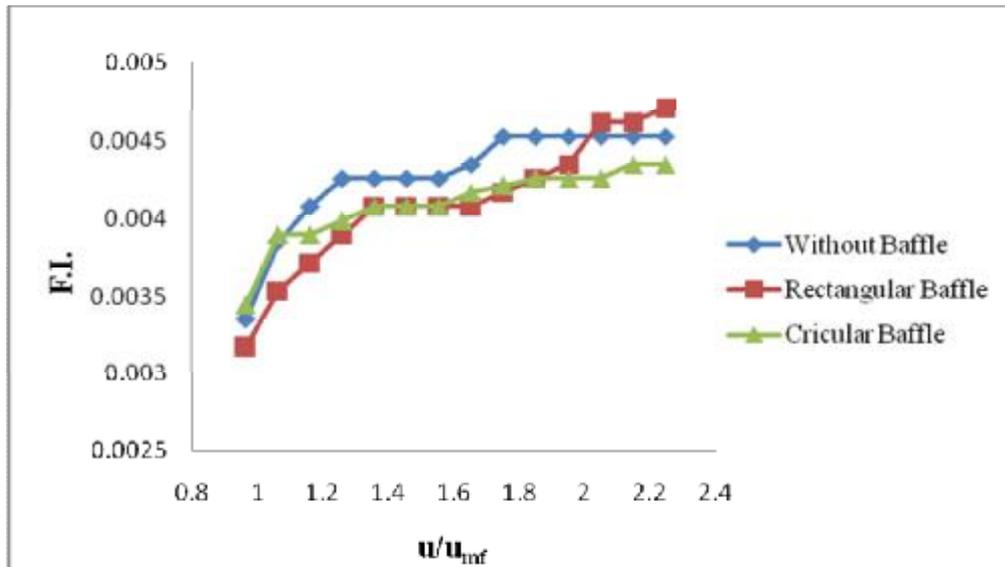
Figure (24) The variation of F.I. with velocity ratio  $u/u_{mf}$ ,  $dp=775\mu m$ ,  $H_s=0.3m$ .
