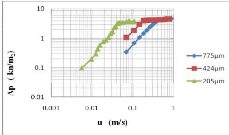
Figure (5) The relationship between the bed pressure drop and the superficial air velocity for different particles diameter, with rectangular baffles column,  $H_s=0.4m$ .
