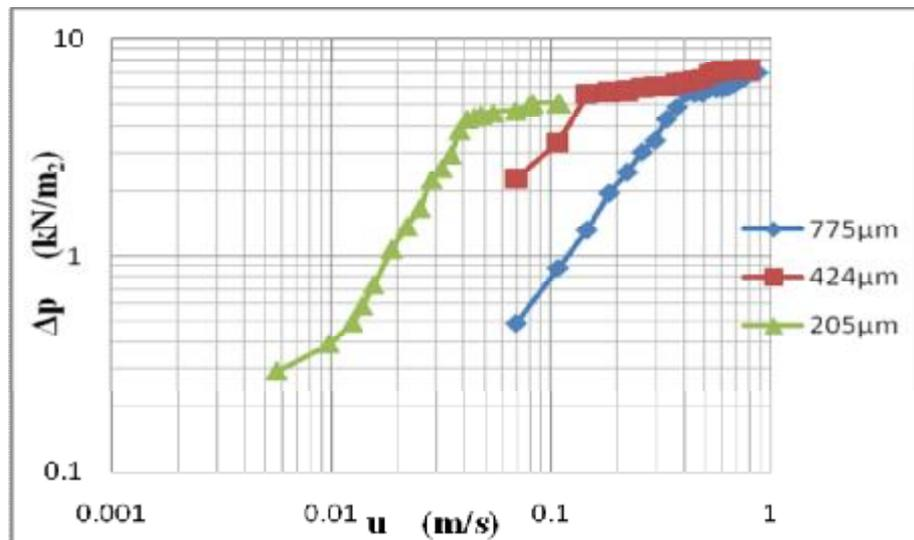
Figure (4) The relationship between the bed Pressure drop and the superficial air velocity for different particles diameter, with rectangular baffles column,  $H_s=0.3m$ .
