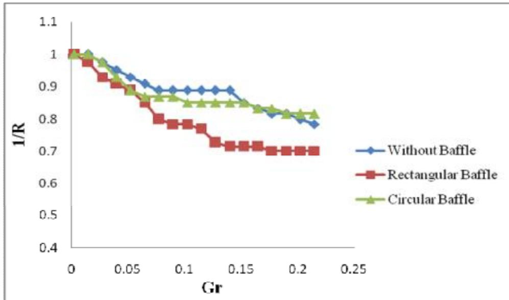
Figure (11) The variation of the reciprocal of bed expansion ratio with mass velocity ratio for baffled and unbaffled beds,  $d_p=424\mu\text{m}$ ,  $H_s=0.4\text{m}$ .
