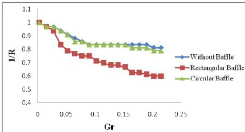
Figure (10) The variation of the reciprocal of bed expansion ratio with mass velocity ratio for baffled and unbaffled beds,  $d_p=424\mu\text{m}$ ,  $H_s=0.3\text{m}$ .
