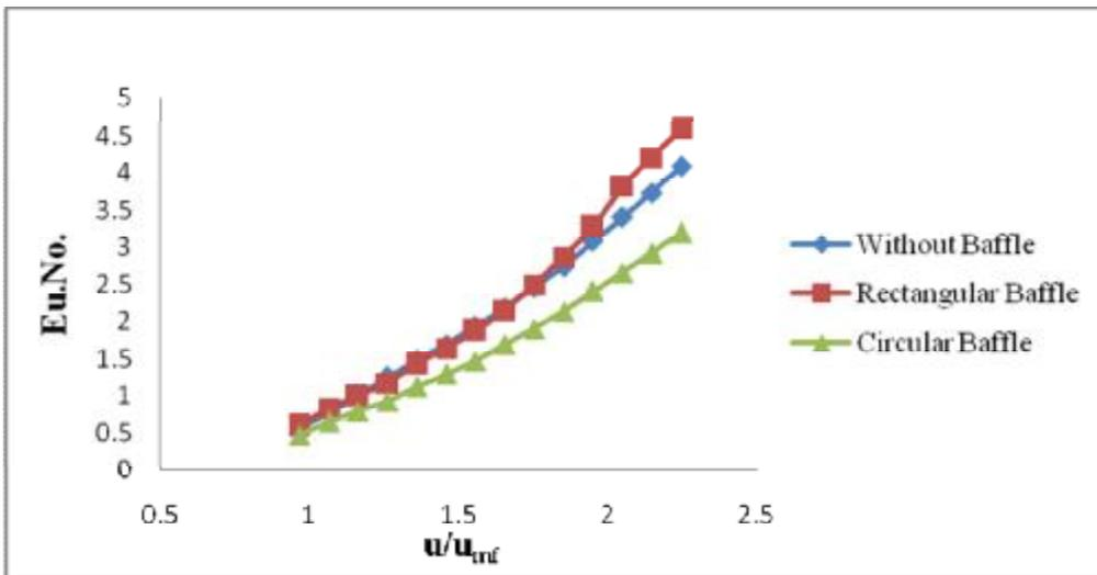
Figure (19) The relation between Eu.No. and velocity ratio  $u/u_{mf}$  for  $dp=775\mu m$ ,  $H_s=0.4m$  fluidized bed.
