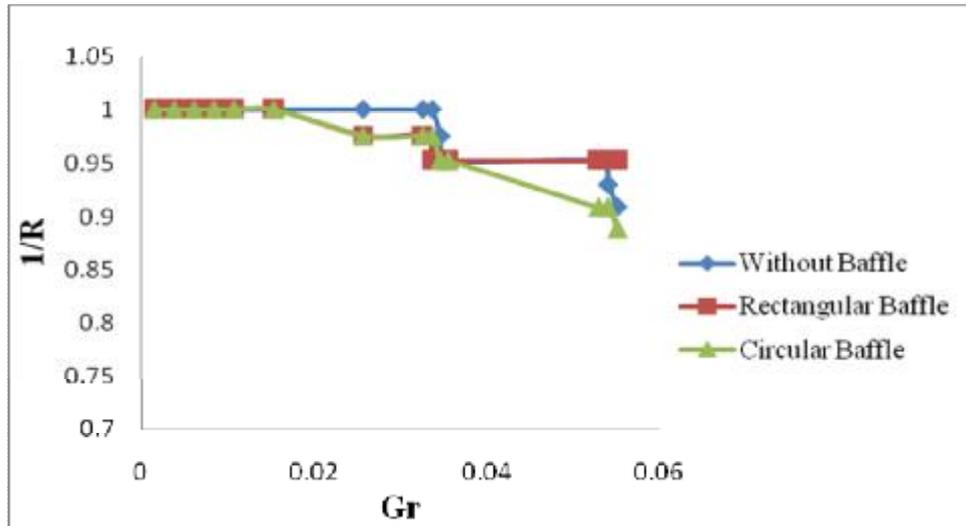
Figure(9) Variation of the reciprocal of bed expansion ratio with mass velocity ratio for baffled and unbaffled beds,  $d_p=205\mu\text{m}$ ,  $H_s=0.4\text{m}$ .
