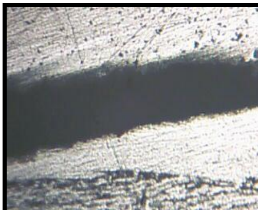
Figure (13) tunnel defect during FSW at 10 mm/min welding speed.
