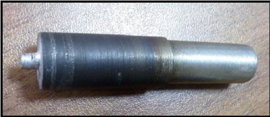
Figure (1) Photograph Picture of friction stir welding tool.
