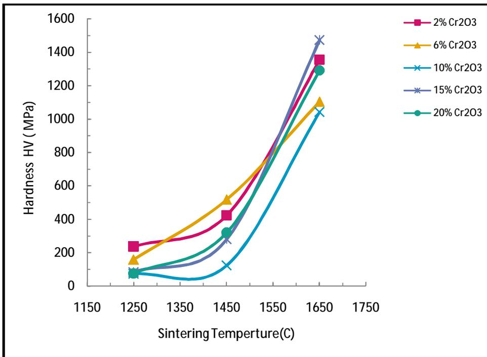
Figure (5) Vickers microhardness for the sintered Al<sub>2</sub>O<sub>3</sub>- %Cr<sub>2</sub>O<sub>3</sub> compacts versus sintering temperature.
