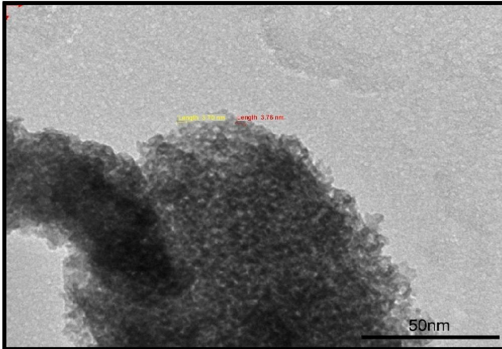
**Figure (1) TEM image for prepared nanocomposite powder after calcination at 600°C for 2 hrs and with 15% Cr<sub>2</sub>O<sub>3</sub>.**
