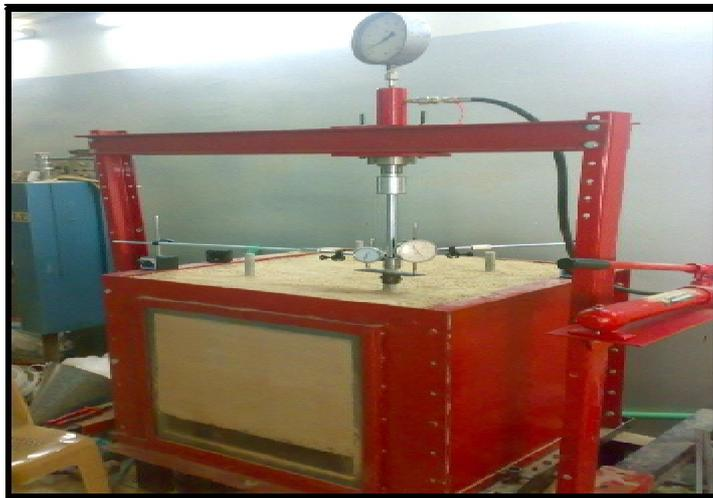
Figure (2) Setup formulation simulated to pile load test.
