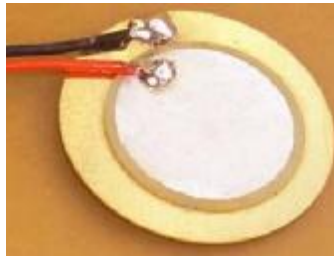
Figure (4) The piezoelectric sensor (Diameter = 15mm).
