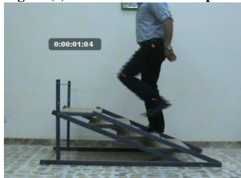
Figure (4) Foot clearance phase.
