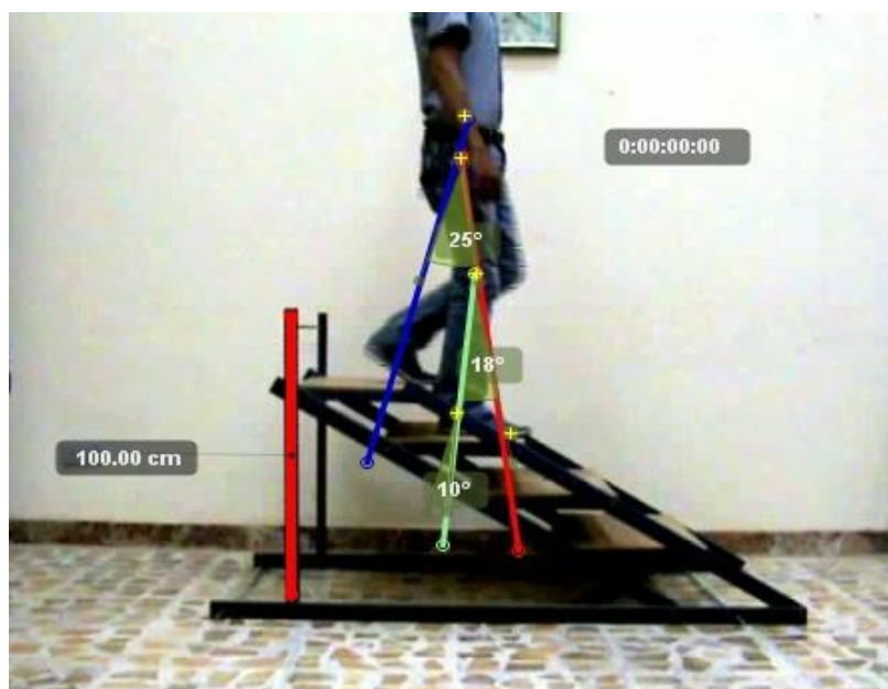
Figure (12) the experimental set-up and the angles arrangement a video camera recorded the spatial positions of Circular passive markers.
