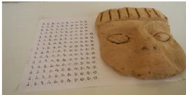
Figure (4) Artificial object with coded targets.
