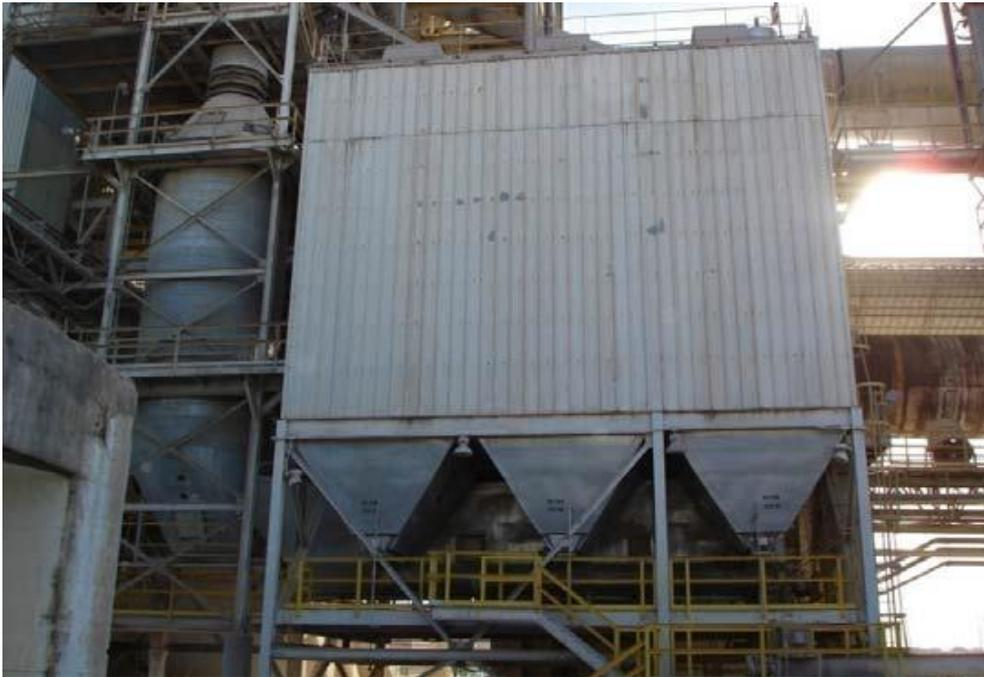
Fig. (1): Dust control device (Courtesy of Capitol Cement
