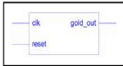
Figure (2) RTL part of Gold code generation.
