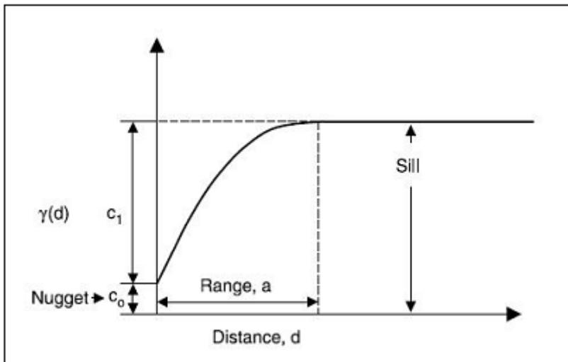
**Figure (1): Typical Parameters of a semivariogram.**
