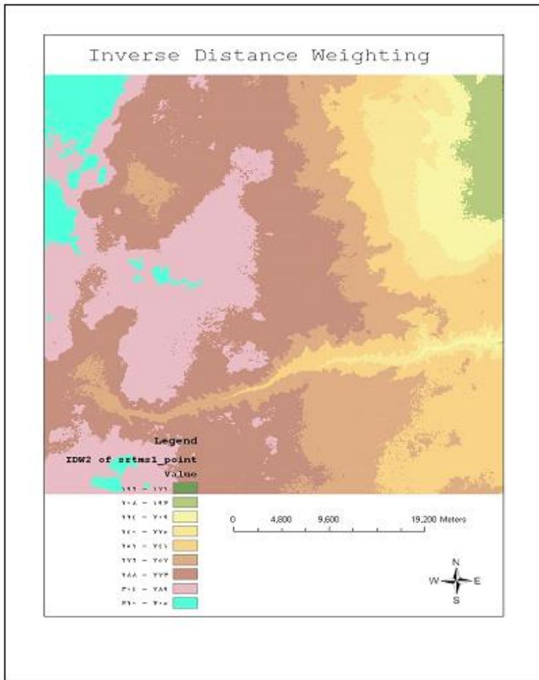
**Figure (5): Surface produced using IDW method.**
