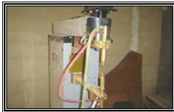
Figure (4) photography of spot welding equipment.
