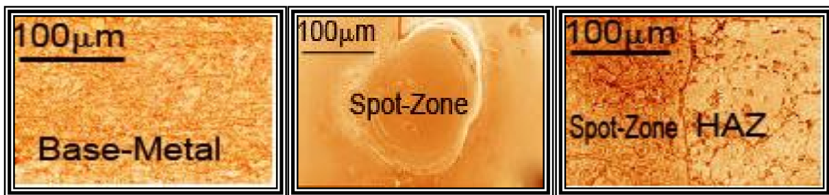
(a) Base metal (b) Heat affected zone (c) Weld metal
