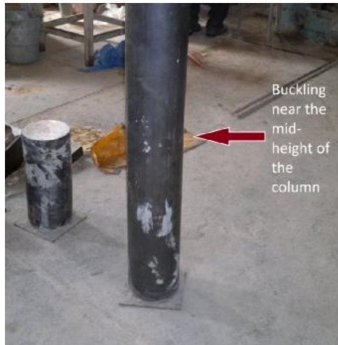
Figure. 10 Failure of the long column
