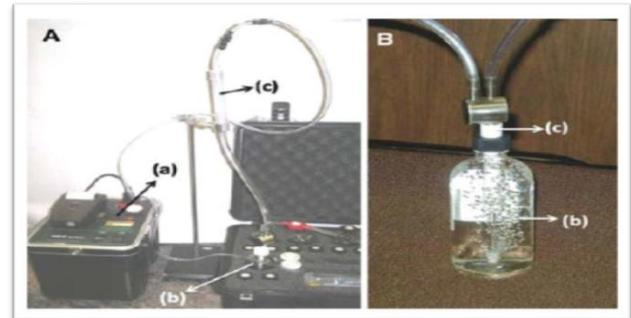
**Fig.(2): Schematic presentations of radon-in-air monitor RAD-7[11].**
