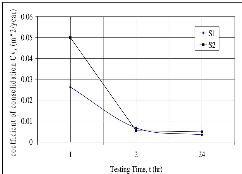
Figure (9): Effect of LID on values of the Coefficient of consolidation, Cv.
