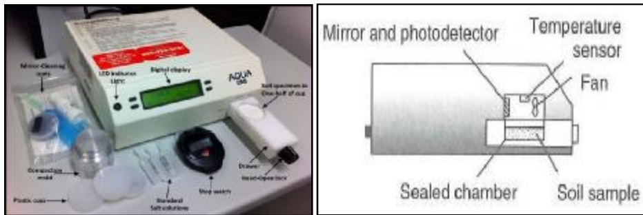
(a) (b) Figure (2) Chilled-mirror hygrometer device, a. photo, b. schematic diagram.
