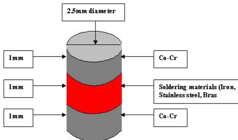
Figure (1): Biocompatibility sample
