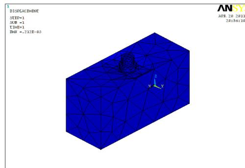
Figure (3): A 3D finite element model of implant and bone block constructed by ANSYS V.12 for FE analysis
