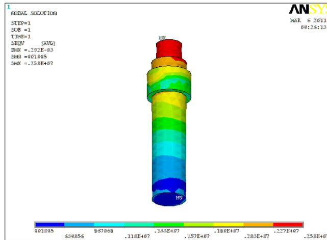
Figure (5): Stress values and distribution along implant-bone interface, the length is 13mm.,the diameter is 3.75mm.
