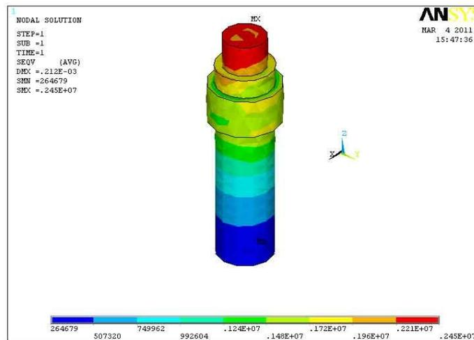
Figure (4): Stress values and distribution along implant-bone interface, the length is 11mm.,the diameter is 3.75mm
