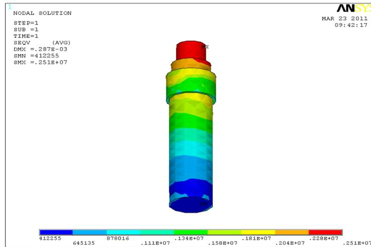
Figure (7): Stress values and distribution along implant-bone interface, the length is 13mm.,the diameter is 4.25mm.
