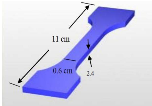
Figure (2) tensile specimen coupon dimensions centimeters.
