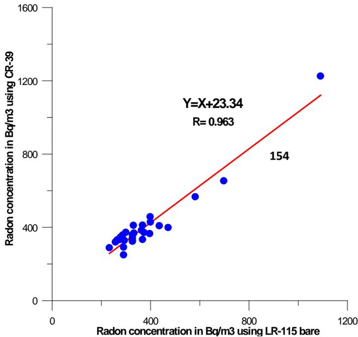
Figure 2. Correlation between Cr-39 and LR-115 type II measurement of radon concentration
